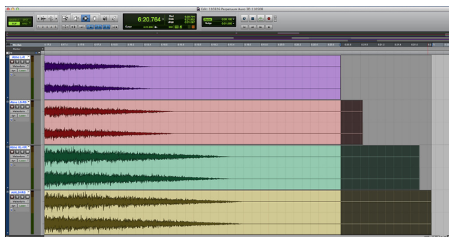
Figure 4: An Auro 3D 8.0 atmosphere sound can be generated from mono or stereo far-away sounding city noise by channel duplicating and mutual time delays of up to 1s.
