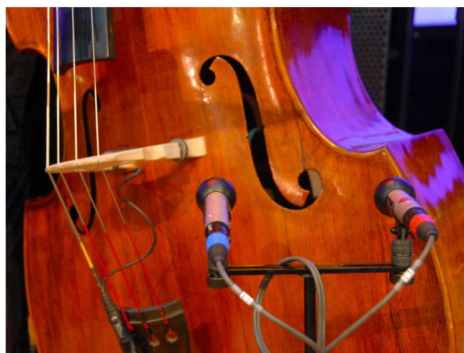
Figure 2: Recording of a double bass by a small AB spot microphone system: The resonating body seems to sound as an own room.
