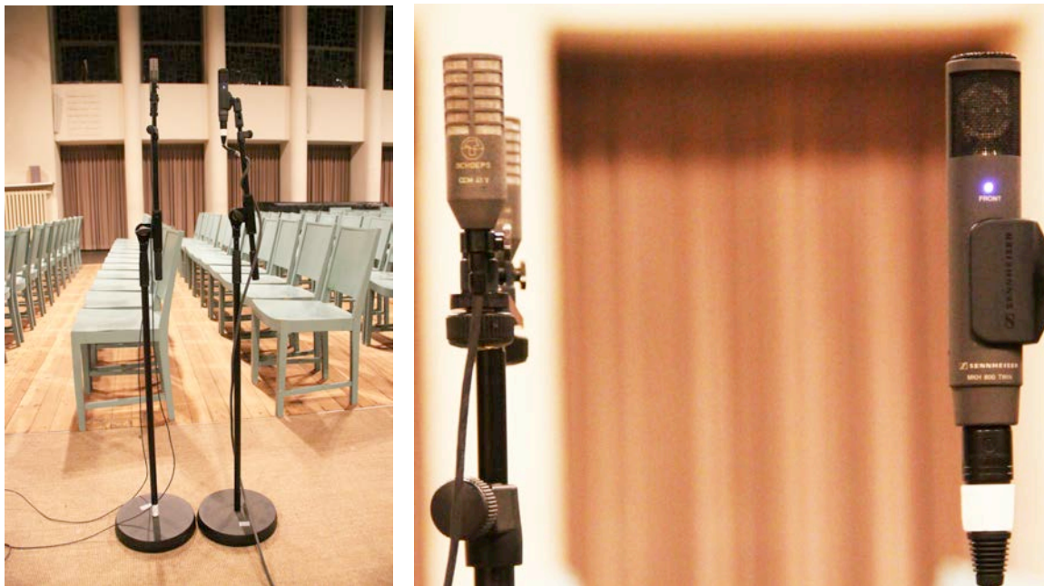
Fig. 6a and 6b: Experimental arrangement of Schoeps CCM-41V and Sennheiser MKH 800 TWIN supercardioids in the Jesus Christ Church in Berlin-Dahlem
