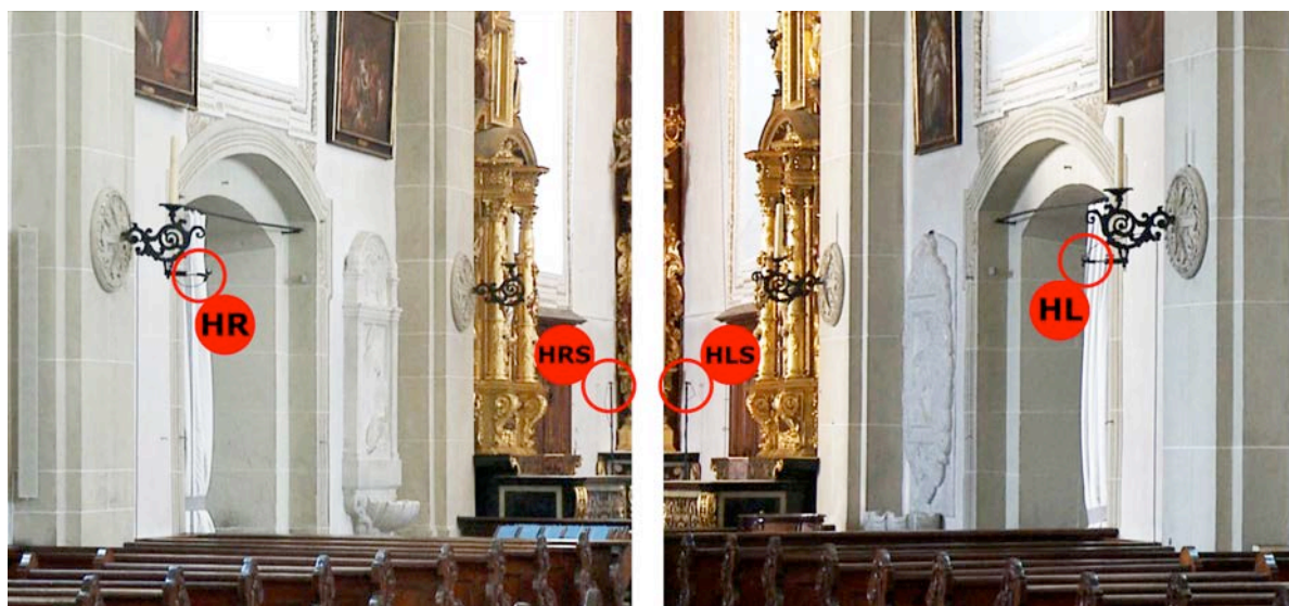
Fig. 4: Microphones in the side aisles with large AB systems in the Hofkirche Luzern, CH
